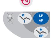
After the instruments have been flushed at high Oxygenal concentration, the start of the dwell time is indicated by a signal tone lasting 4 sec. The dwell time is 30 min. During this time, the unit can be switched off. After the end of the intensive disinfection, the Unit ON LED and the Service LED flash. After the instruments have all been replaced, the unit is ready for operation again.
