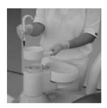
Fill Oxygenal (max. 1 litre). If a signal tone is heard at one second intervals (10 tones), the storage tank is full. Stop filling immediately.
